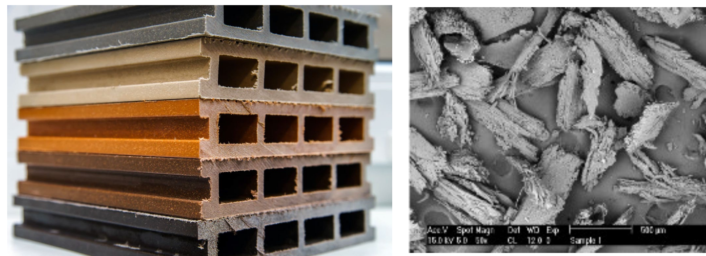
Figure 1. Left side – WPC profile – floor, right side – SEM of sawdust (Atuanya and Ibhadode, 2011)
