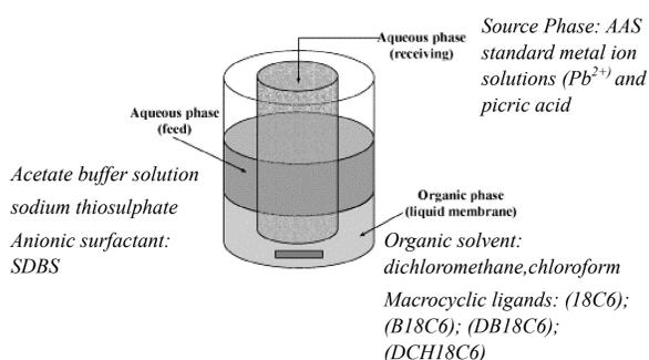
Figure 2. "Transport cell" used for the experiment
