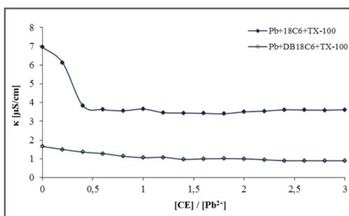
Figure 4. Influence of crown ether structure on the conductivity of 3-component systems: Pb<sup>2+</sup> - TX-100- CE (DCM)
