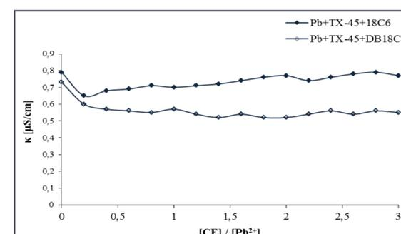
Figure 7. Influence of crown ether structure on the conductivity of 3-component systems: Pb<sup>2+</sup> - TX-45- CE (1,2-DCE)
