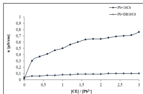
Figure 2. Influence of crown ether structure on the conductivity of 2-component systems: Pb<sup>2+</sup> - CE (DCM)
