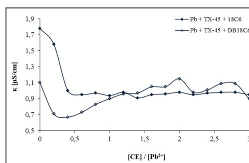
Figure 6. Influence of crown ether structure on the conductivity of 3-component systems: Pb<sup>2+</sup> - TX-45- CE (DCM)
