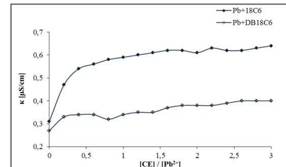
Figure 3. Influence of crown ether structure on the conductivity of 2-component systems: Pb<sup>2+</sup> - CE (1,2-DCE)
