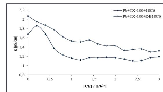
Figure 5. Influence of crown ether structure on the conductivity of 3-component systems: Pb<sup>2+</sup> - TX-100- CE (1,2-DCE)
